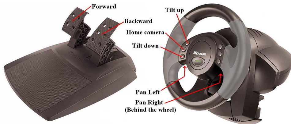
Figure 5.5: The Microsoft Sidewinder Wheel and pedal and the controls used for the experiment.
